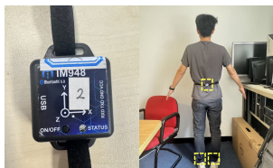
Fig. 14. Wireless IMU(left) and mounting location(right).
