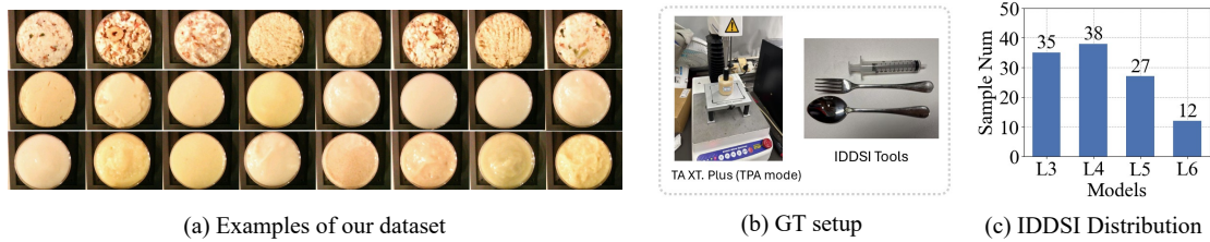
Fig. 9. The setup of the evaluation. (a) Partial examples of our dataset. (b) The setup of of ground truth. (c) The IDDSSI level distribution of our dataset.
